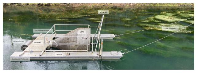
Figure H-1. Labelled image of a rotary screw trap showing parts and terminology.
